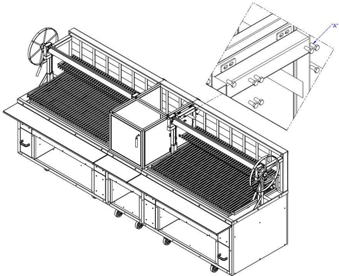
“A” Align and tighten the screws.
