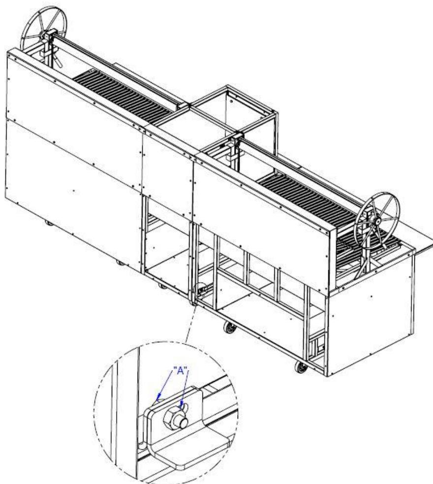
“A” Align and tighten the screws (8x).
